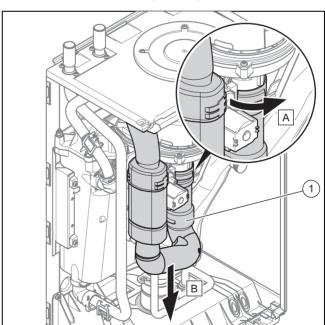
4. Remove the air intake pipe (1).
